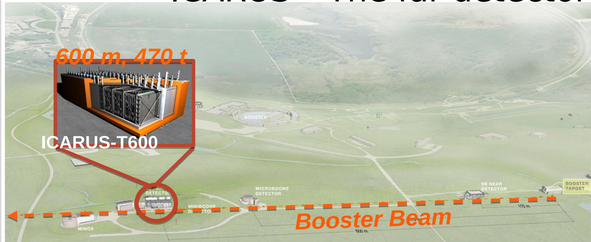
Given its large mass and relatively large distance from the source the ICARUS-T600 will have high sensitivity to neutrino oscillation effects.
