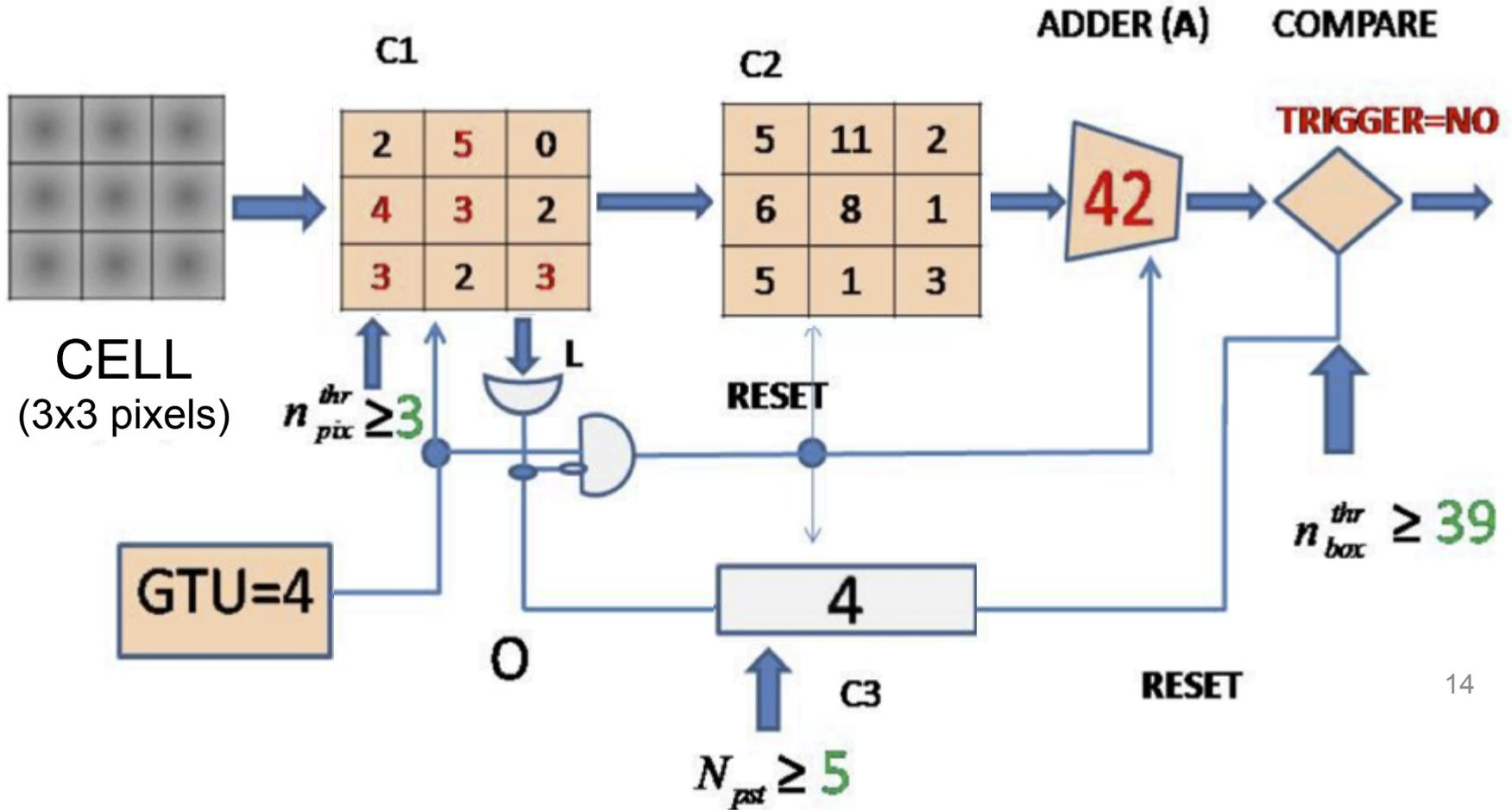
Local threshold:  $N = 3$  photoelectrons (in 1 pixel)
