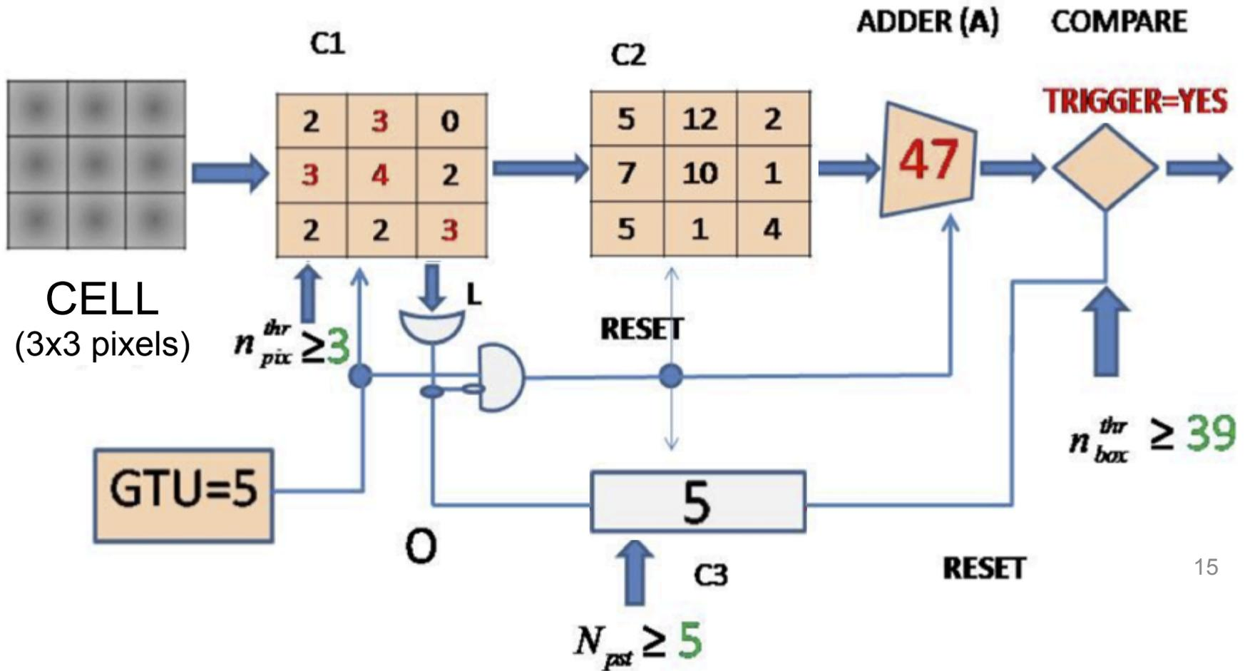
Series of tests of the internal Level1 trigger at the level of 1 elementary cell (EC)
