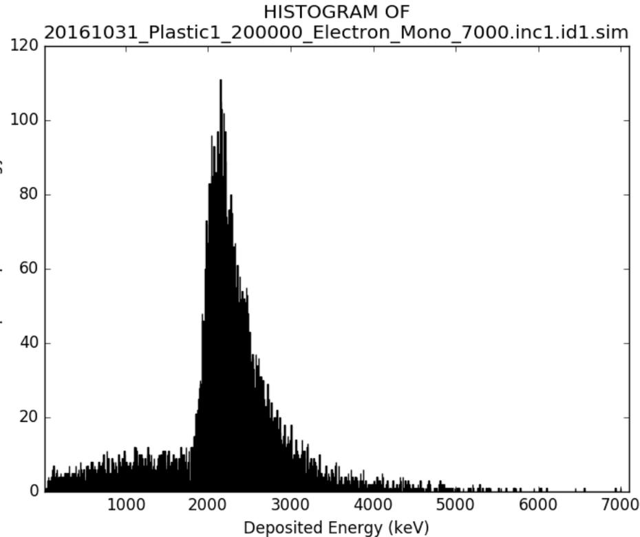
Scintillator: BC-412, thickness: 6.2 mm.
